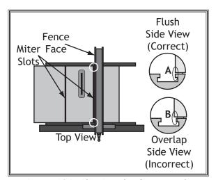
**Figure 106.** Aligning the fence to the miter slot.
